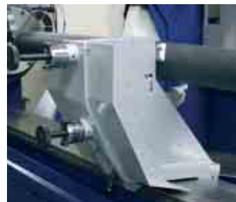
Steady rest capacity Ø30-180 mm
