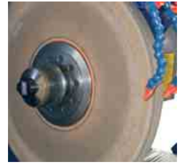
Automatic balancing system for grinding wheel - incl. display
